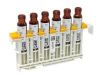
Up to six quality controls can be loaded on a single rack and up to four racks can be loaded on the instrument.
